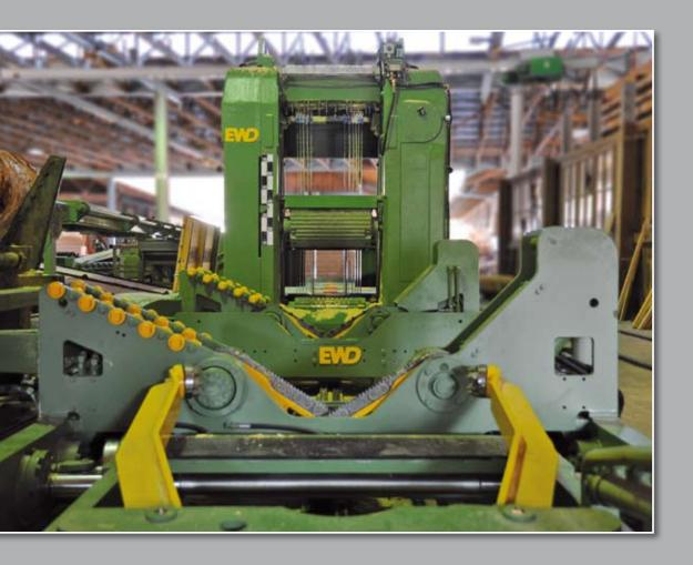
Universal fast infeed carriage system, remote controlled
