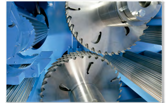
Double arbor circular saw with lumber guides
